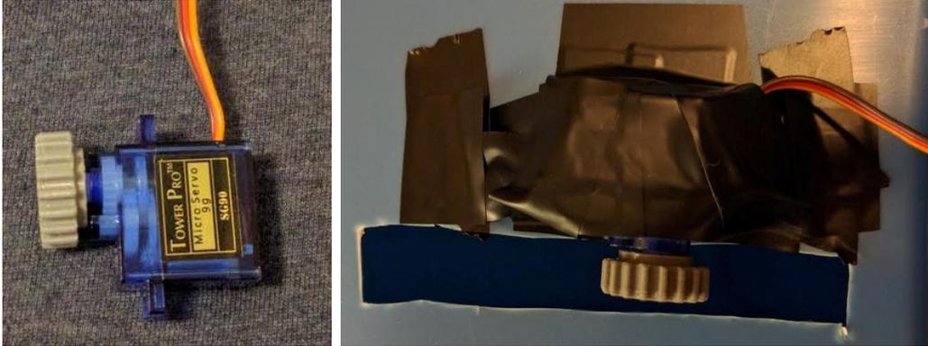
After getting the servos in place, I had to wire everything. I decided that the servos would be triggered using pushbuttons. I used an Arduino Mega to program my circuit and a lot of electrical tape to hold everything in place. I used a 9V power supply to power my circuit.
